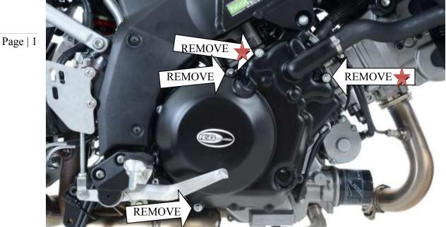
In this kit there should be: 1 x Engine Case Cover (PC0175). 2 x M6 x 40mm long button head bolts (rear). 2 x M6 x 75mm long button head bolt (mathematication). 4 x M6 washers.
