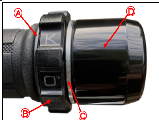
A — Plastic Thrust Washer B — Friction Nut & Grub Screw C — Kaoko bar-end Body D — OEM bar-end weight
