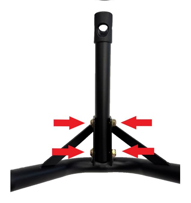
STEP 4 PLACE THE GOLD BOLTS WITH THE SUPPLIED WASHERS THROUGH THE SUPPORT BAR AND USE THE NUTS TO TIGHTEN INTO PLACE. (ENSURE THE PIN HOLE IS FACING THE SAME DIRECTION AS SHOWN)
