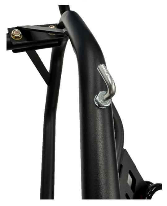
STEP 7 INSERT THE CALIPER HOOK INTO THE SIDE OF THE STAND BY HAND AND THEN ADJUST TO THE CORRECT ROTATION BY ADJUSTING THE NUT. (TRY TO HAVE THE HOOK FACING UPWARDS WHEN THE STAND IS IN USE)
