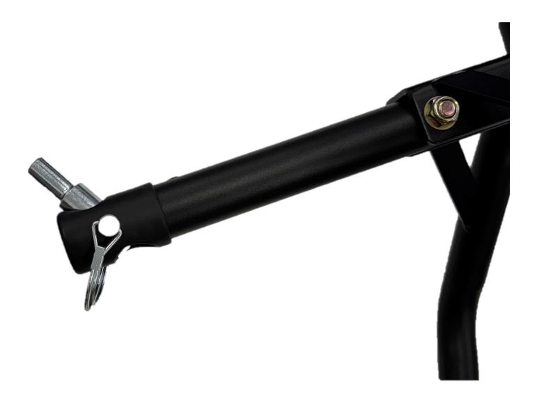
STEP 6 PLACE THE HEAD STOCK PIN THAT IS MADE TO FIT WITHIN YOUR BIKES HEADSTOCK HOLE IN THE BOTTOM OF THE FORK CLAMP.
