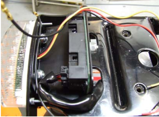
CONNECTING BLOCK IN POSITION
